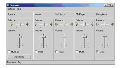
7. At the bottom of the Microphone section, click the *Mute* box in the *Microphone* section to prevent the Microphone directly feeding back its own audio to the earpiece (i.e. "sidetone").
