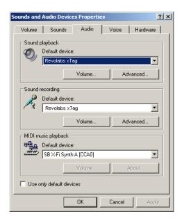
4. Open the *Volume* settings for *Sound recording* to view the volume levels selected for the microphone input (*Capture*) on the computer.
